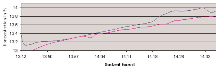
The time lag generated by sensors concepts that require a bypass results in process regulation imprecision.
