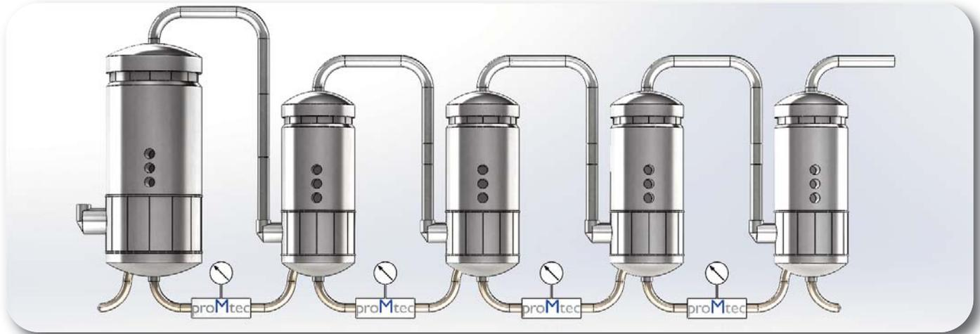
In the multi-stage evaporating station the thin juice is thickened to the required maximum dry substance content. In the stage of evaporation thermal efficiency aiming at energy saving is also of major economic importance for processes in the subsequent crystallization.
