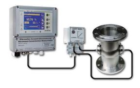
The contactless measurement consists of two flat sensors that are fitted in a pipe, a temperature sensor to compensate temperature fluctuations, a microwave module and the evaluation unit.
