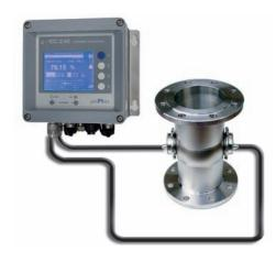
The contactless measurement consists of two flat sensors that are fitted in a pipe, a temperature sensor to compensate temperature fluctuations and the evaluation unit.
